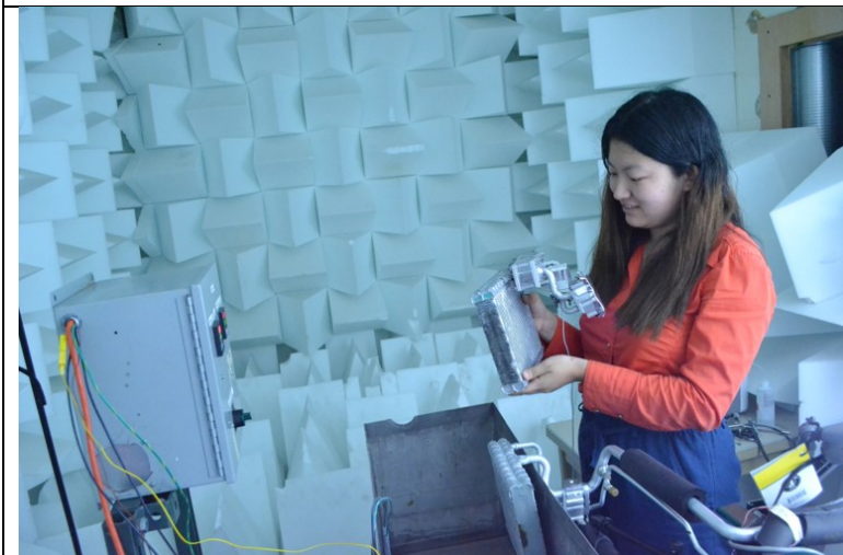
Setting up an experiment to study flow induced noise in automotive air conditioning systems
