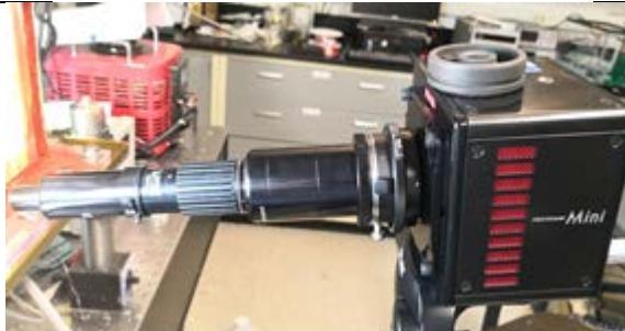
A black Photron FASTCAM Mini AX 200 high-speed camera mounted on a tripod. The camera body is black with red and white markings. A long, thin lens is attached to the front. The background shows a laboratory or workshop setting with various equipment and supplies. |
